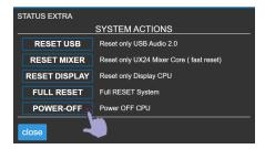
This feature does not completely turn off the console. Full shutdown is done from the mechanical on/off switch. Once the CPU shut down, wait a few seconds before turning off the power switch.
