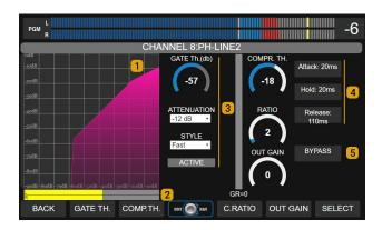
The DYNAMIC stage has a noise gate and dynamic compressor. Processor settings can be saved in the current scene (see SCENES screen).
