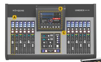
**B** A main touch screen, from where certain functions are controlled: audio processors, "virtual" channels (channels not assigned to real faders), simplified functions for telecommunications, scenes. This screen also contains the level meters, clock and counter.
