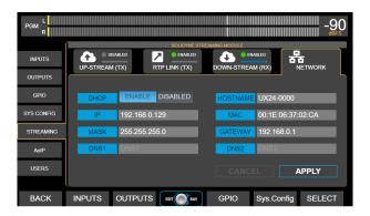
Network settings for the **UX24 streaming module**. At the present version this settings are fixed and depends on the settings of the LAN (DHCP).
