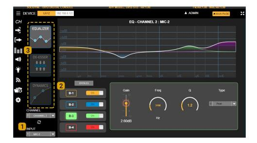
From the PROCESS screen you can access the controls of the equalizer, the de-esser and the dynamic compressor. Its use is similar to that described for the on-board display (see 3.7 Audio processes).
