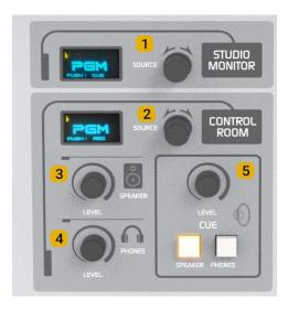
In this section the operator assigns the signals that will be heard on the monitor speakers and the headphones of the Studio and Control Room.
