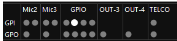
OXYGEN REMOTER displaying of the activated GPI 3
