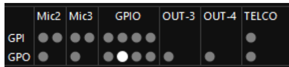
OXYGEN REMOTER displaying of the activated GPO 3
