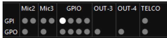
OXYGEN REMOTER displaying of the activated GPI 2
