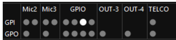
OXYGEN REMOTER displaying of the activated GPI 4
