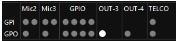
OXYGEN REMOTER displaying of the activated OUT 3 GPO
