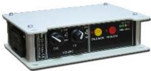
Battery powered, belt pack style unit with a single talkback circuit
