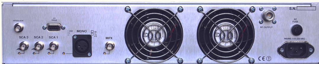
REAR SIDE WITH STEREOCODER BUILT IN
