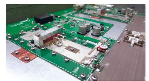
2 planar design RF pallets each of 1.25 kW
