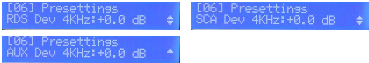
Fig. 5.34 – Presetting auxiliary channels deviation adjustment
