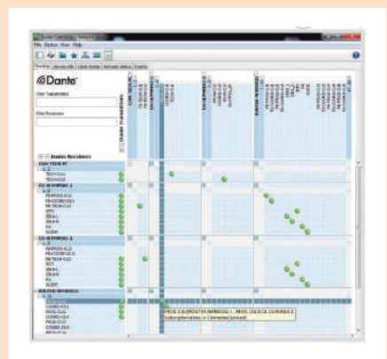
Figure 3. Netbox 32 configured with Dante Controller in order to communicate with three Olympia 3 commentary units.
